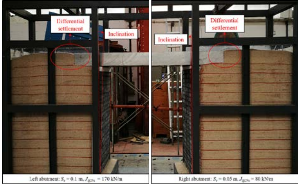
Fig. 22. Photos of the left and right GRS abutments after the completion of the shaking test (T1)
