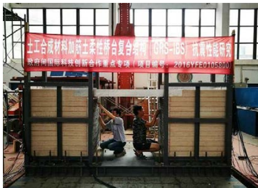
Fig. 20. The completed GRS-IBS model before applying the dynamic load
