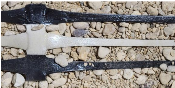
Fig. 1. A transmission line sensor-enabled geogrid placed in soil within the testing shear box prior to loading.
